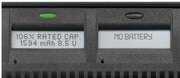
Display shows battery capacity, voltage, charge status and more, in real time.
